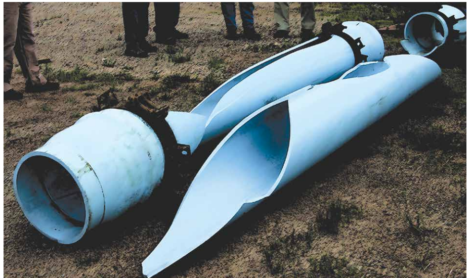
The contractor exposed the pipeline to find that the pipe had failed.
